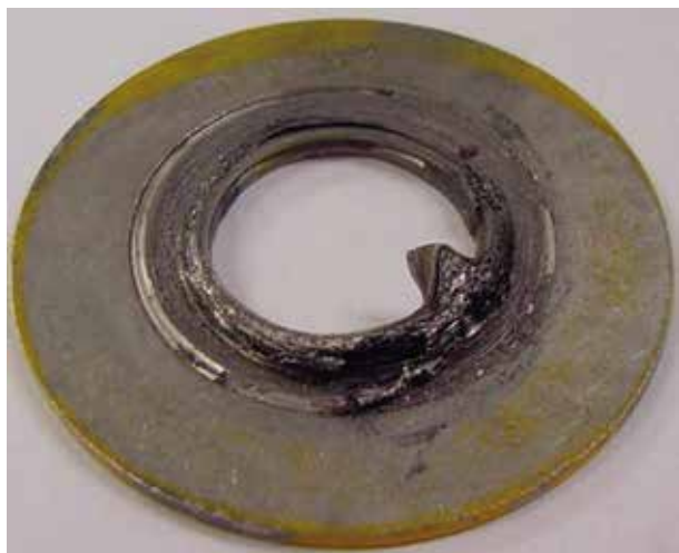
Figure 3. Buckled standard spiral wound gasket from small bore, slip on flange.
