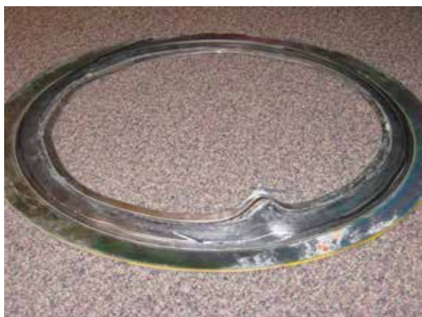
Figure 2. Buckled inner spring spiral wound gasket.
