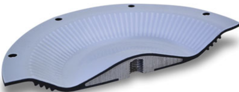
Figure 4: Cross-section of an integral piston diaphragm (IPD) consisting of a PTFE face, fabric reinforced rubber backer and integrated piston to attach directly to the pump shaft.
