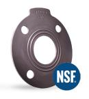
gasket incorporates raised ribs that concentrate the loading force and enable a seal with less torque than expanded PTFE gaskets; a key benefit given the torque limitations on PVC, CPVC, FRP, and other non-metallic flanges.
