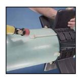
8. Re-insert Slide-Locks completely into segments by lightly tapping Slide-Lock back into position.
