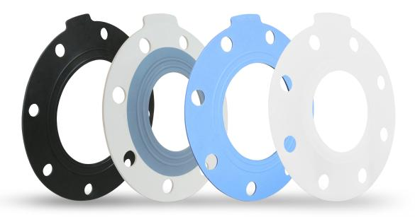
The STRESS SAVER® family of products have provided reliable sealing performance in low load flanges for decades. The raised rib features are key in achieving stress optimization through reduced contact area in non-metallic flanges where torque and stress are limited. Each of the STRESS SAVER® styles are designed to meet a critical need whether that is chemical resistance, high purity sealing or compatibility with piping polymers of construction.
